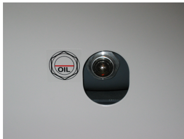
Compressor - oil level
