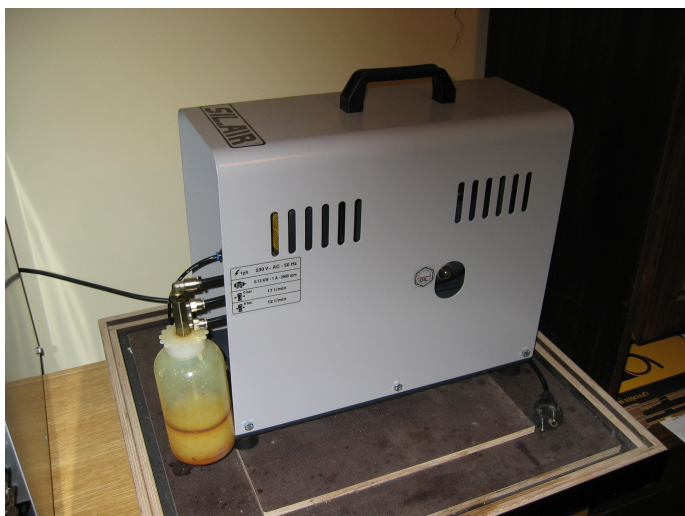
Compressor with drain bottle
